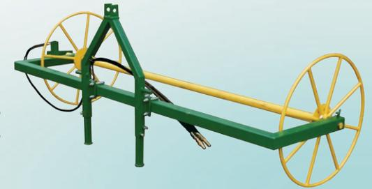
Zwijarka / Foil-rolling machine / Plastindragning
